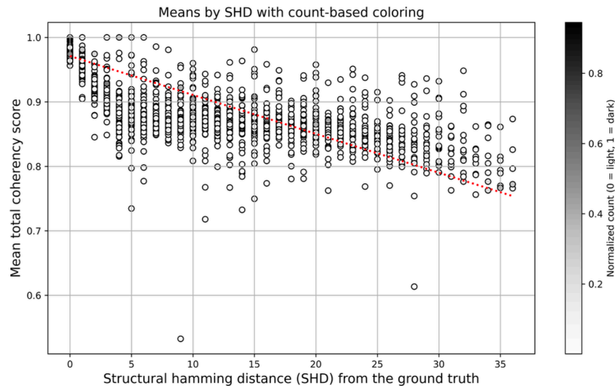
Figure 6: We generated 127000 data sets from 127 ground truth DAGs with 4 to 10 nodes from sparse to fully connected. In this plot, we show the 127 means each over 1000 DAGs with the same configuration. The red dotted line shows the weighted regression of the mean scores over 1000 random DAGs each on the SHD weighted by their counts.
